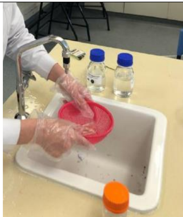
Figure 6. Separating the HCl solution from the CaCO 3 strips.
